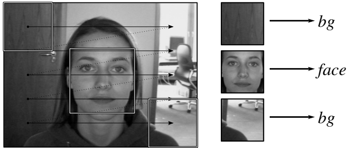
Fig. 1. Scanning the image with a classifier. Individual sub-images of the image are classified by a classifier (Image source: BioID dataset).
